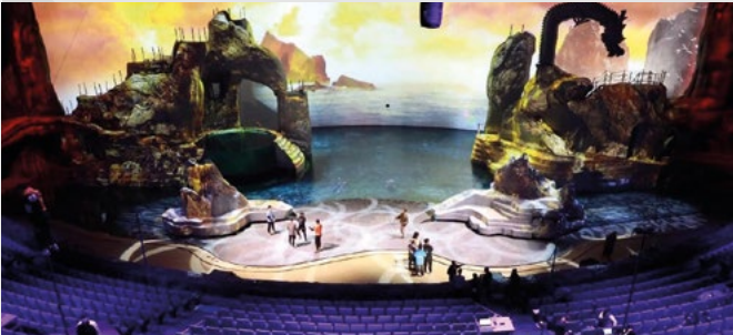
↑ A set of inflatable spheres is one of the dominants of the 50 m wide water stage in Qing Show theatre. Some of the spheres move during performances thanks to an underwater track-based construction.
